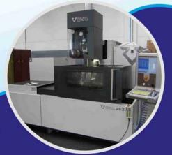
EDM area, die sinking and wire cut machines. Precision boring machine for holes from 0,15 through 3 mm.
