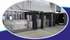
Semiautomatic F.P.I. equipment with 700 x 800 x 800 mm tanks capacity and operating to ASTM 1417 (IA3, ID2, ID3). Posted personnel qualified according to NAS 410
